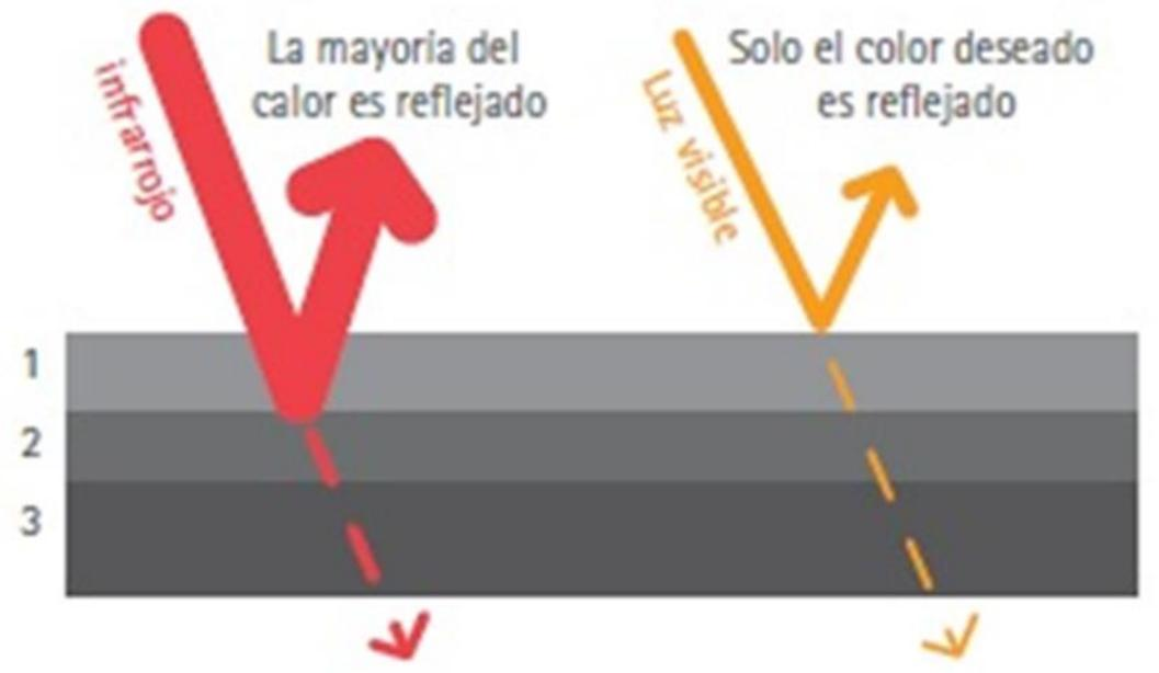
\* COATING ANTI-UV - MEMBRANA IMPERMEABLE COOL COLOUR - SOPORTE
